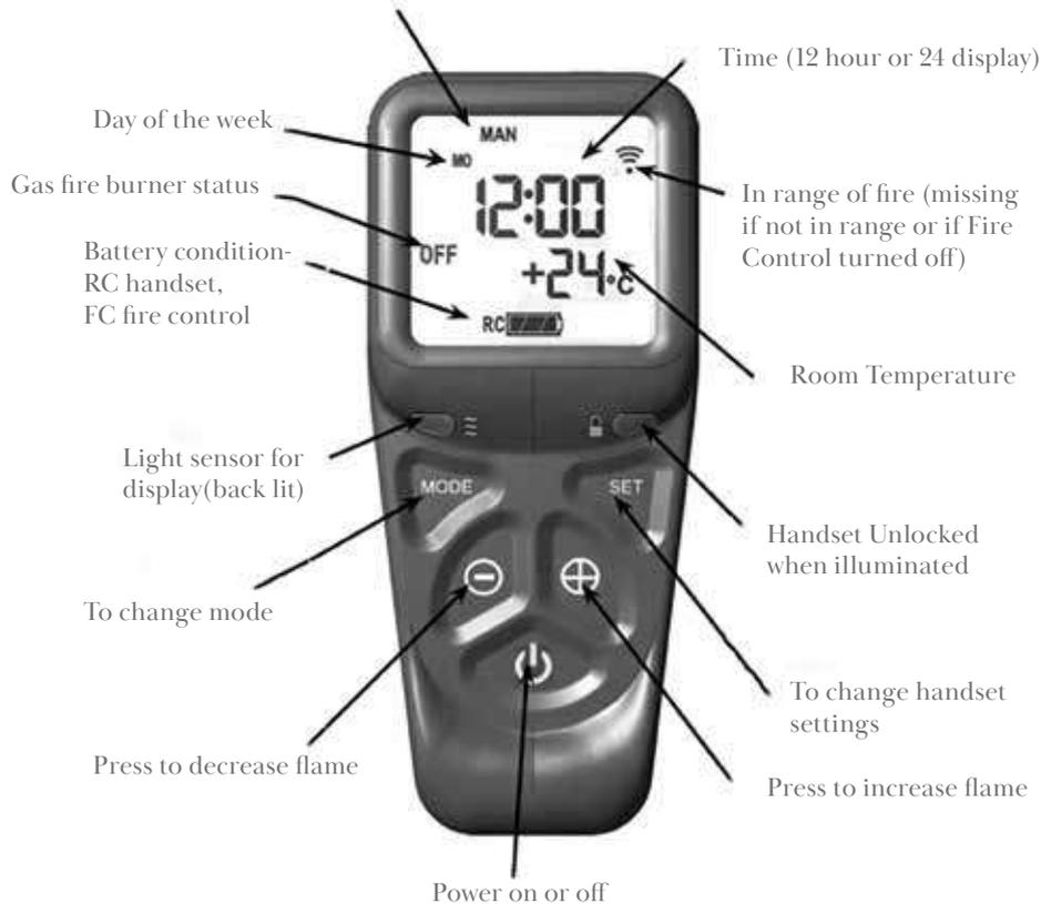
Fig.4 Remote control handset
