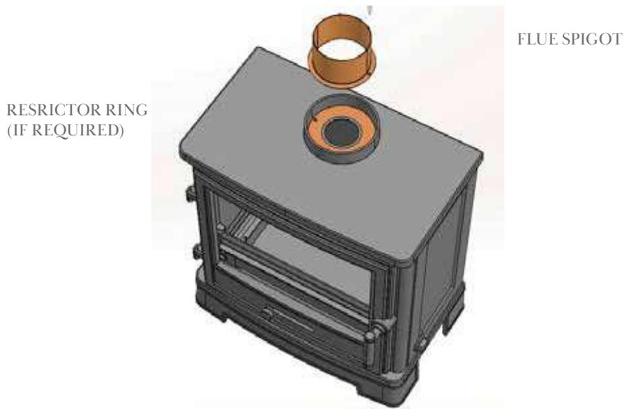
Fig.7 Flue connections
